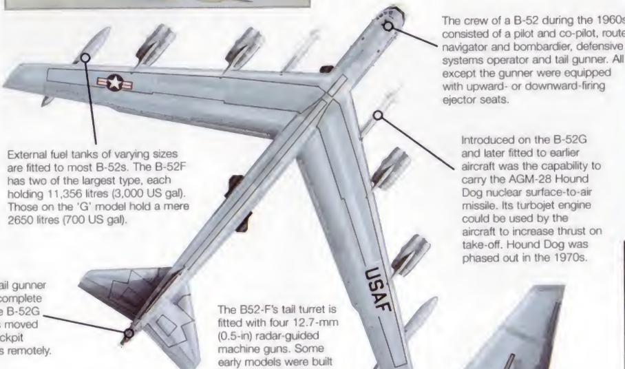
B-52s carry an enormous amount of fuel – around 147,112 litres (38,863 US gal) – in large internal tanks in the fuselage and wings. The J57-powered models also carry water tanks for the water injection system used by the engines during take-off to increase thrust.
